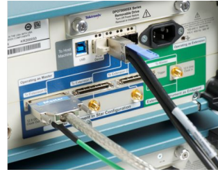
UltraSync connection on instrument with Master role
