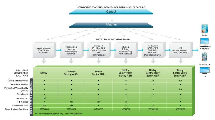
Medius<sup>™</sup> offers video service providers an effective way of managing and aggregating status, alerts, and reports from multiple Sentry<sup>®</sup>, Sentry Verify<sup>™</sup>, and Sentry Edge<sup>™</sup> units deployed throughout a network.
