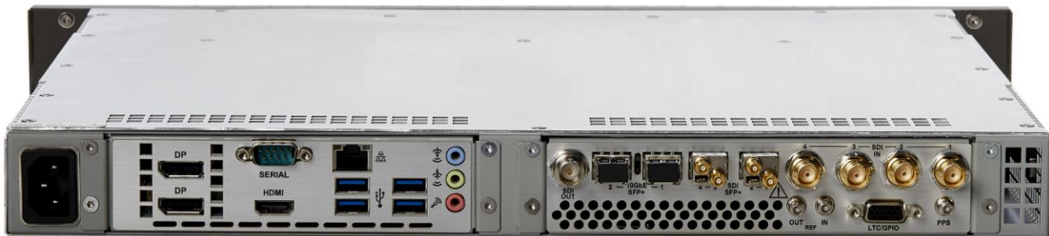
MPX2-10 front and rear panels
