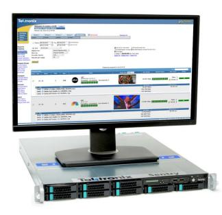
Sentry Verify<sup>™</sup> monitors and validates MPEG Transport Stream quality at hub sites as an integral part of the source-to-edge monitoring solution.
