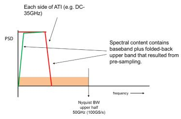
Figure 11. Signal on each leg of the ATI channel.
