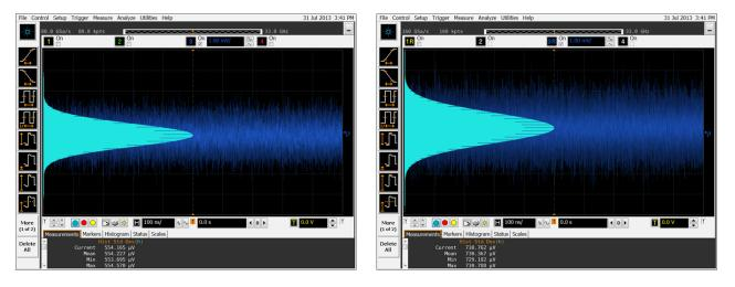
Figure 9. Noise performance comparison of Keysight DSAX95004Q oscilloscope channels (standard vs "RealEdge").
