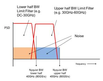
Figure 8. Noise Power Spectral Density across Nyquist bandwidth.
