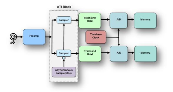
Figure 10. Asynchronous time interleave circuit.
