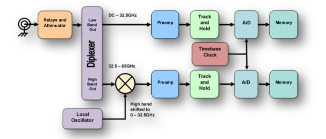
Figure 5. Example of a mixer-based acquisition channel.
