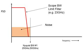
Figure 2. Random noise power spectral density (PSD), relative to frequency.
