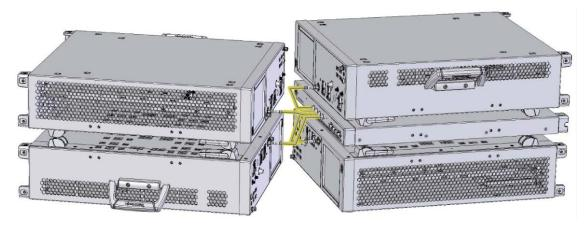
Figure. 7: Graphical depiction of two DPS70000SX units and an OM4245 Optical Modulation Receiver positioned face-to-face for 400G coherent optical modulation applications.
