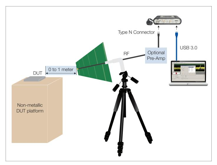
Figure 8. Block diagram of pre-compliance radiated emissions test setup.
