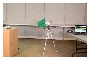
Figure 4. Affordable pre-compliance testing can easily be set up to uncover potential problems so that you can minimize test time in more expensive compliance test facilities
