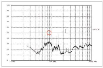
Compliance testing shows a failure around 90 MHz.
