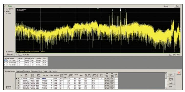
Figure 11b. Test results of DUT. No out of limit conditions were attributable to the DUT.
