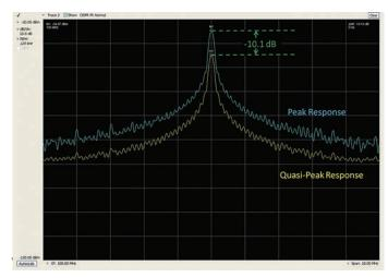
**Figure 6.** Quasi-peak responses will always be less than or equal to peak detection, never larger. So you can use peak detection to do your initial EMI trouble-shooting and diagnostics.
