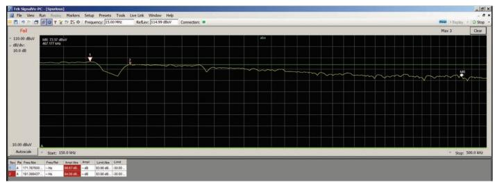
Figure 15. Conducted emissions test showing an over-limit condition at the lower end of the spectrum.
