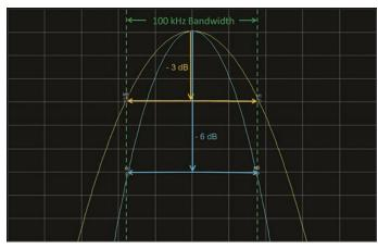
Figure 5. Most EMI standards specify 6 dB bandwidth. Using 3 dB bandwidth will give very different results.
