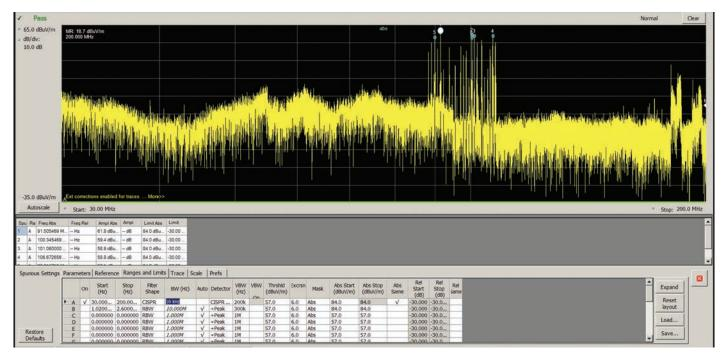
Figure 11a. Environmental background results. Broadcast signals are clearly visible in the VHF band.
