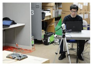
**Figure 7.** Shows our pre-compliance setup located in a basement of one of our buildings.
