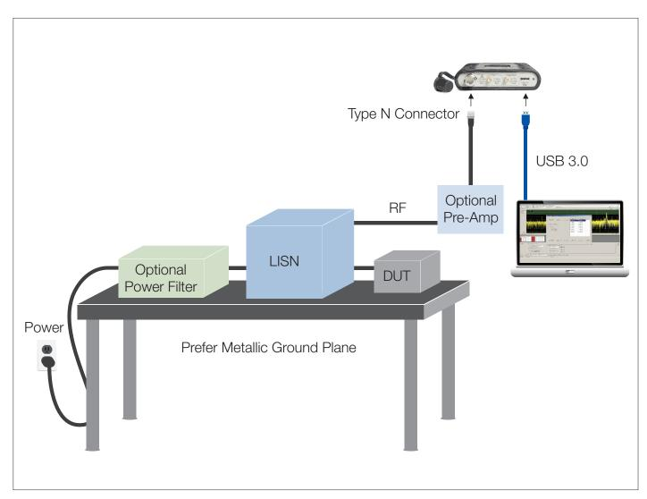
Figure 14. Block diagram of pre-compliance conducted emissions testing.
