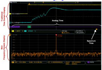
Integrated spectrum analyzer with dedicated acquisition system enables independent control and optimal views of both the time and frequency domains. Spectrum time indicates where in time the spectrum shown came from. Using WaveInspector®, one can easily view and navigate through time correlated analog, digital, and RF.
