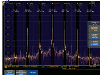
Typical spectrum analyzer measurements are supported, including Channel Power, Adjacent Channel Power Ratio, and Occupied Bandwidth.
