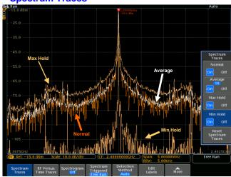
Unlike traditional FFT, the MDO4000C supports typical spectrum analyzer traces: Normal, Average, Max Hold and Min Hold.
