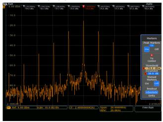
Automatic Markers identify spectral peaks, with the reference marker assigned to the highest amplitude peak. Manual Markers can also be used to investigate other areas of interest in the spectrum or to measure phase noise and noise density.
