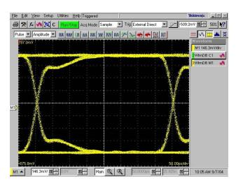
Figure 2. The same signal with the addition of probe loading.
