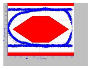
TDSUSB2 USB 2.0 Signal Quality Test Eye Diagram Captured with P6780 Differential Digital Probe using iCapture Analog MUX
