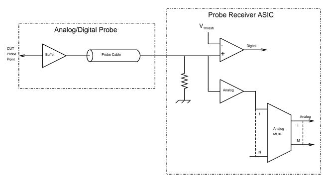
Figure 5. Block diagram of the basic of the analog MUX.
