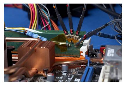
Figure 4. Insufficient room for probing.
