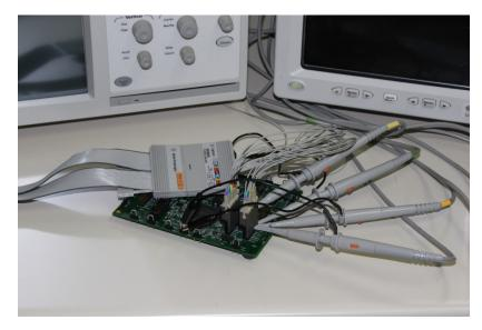
Figure 3. Substandard double-probing.
