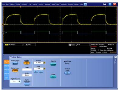
Figure 6. Edge ringing causing digital transitions.
