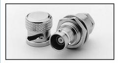
Model 237-TRX-TBC: 3-lug female triax bulkhead connector with cap for assembly of custom panels and interface connections. High voltage rating for use with 7072-HV, etc. Uses miniature coax cable, not triax cable, at soldered end. Bulkhead is outer shield.
