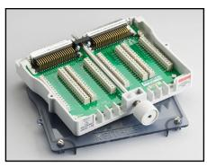
**Model 3732-ST-C:** Screw Terminal Block. Enables screw terminal access and additional matrix sizes including: quad 4×28 (1W), dual 4×28 (2W), single 4×56 (2W), dual 4×56 (1W), and single 4×112 (1W).
