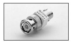
Model 7755 50 $\Omega$  Feed-Through Terminator: BNC-to-BNC adapter for terminating RG58 cable in its characteristic impedance. VSWR <1.1, DC-250MHz.
