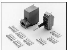
Model 7078-KIT: 38-pin male plug assembly with strain relief and 40 contacts for assembly of custom cable and harnesses compatible with Model 7071 8×12 Matrix Card, Model 7071-4 Dual 4×12 Matrix Card, and 7078-MTR Mass Terminated Receptacle. Requires 7078-HCT; recommend 7078-CIT.
