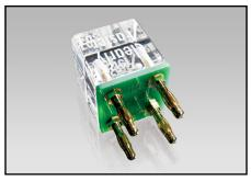
Model 8620 Four-Wire DMM Shorting Plug: Provides a low resistance 4-wire short to both observe and cancel DMM offset resistances and voltages to improve measurement accuracies.
