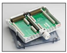
**Model 3732-ST-R:** Screw Terminal Block. Enables screw terminal access and additional matrix sizes including: dual 8×28 (1W), single 8×28 (2W), and single 16×28 (1W).
