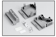
Model 2600-KIT: Screw terminal connector kit with extra screw terminal connector, strain relief, and cover for a single SourceMeter channel (two needed for use with Models 2602B, 2612B, and 2614B).
