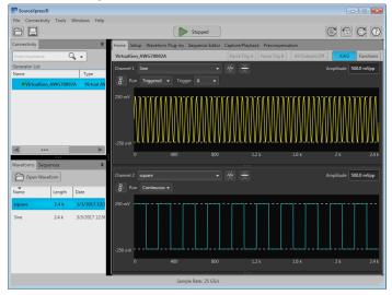
SourceXpress is a PC based software environment that enables Tektronix waveform creation plug-ins, simulates the native environment of a Tektronix AWG70000 or AWG5200 series Arbitrary Waveform Generator, and provides control of a connected generator. SourceXpress allows you to create signals anywhere without being tied to a signal generator. SourceXpress brings a uniform look and feel to waveform creation while enabling an ever growing library of waveform creation plug-ins.
